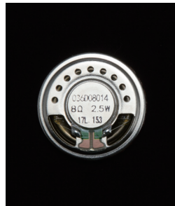
Icom custom high power handling capacity speaker
